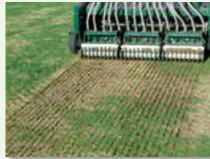
TriWave technology creates optimum slits for improved seed-to-soil contact, while minimizing turf disruption.
