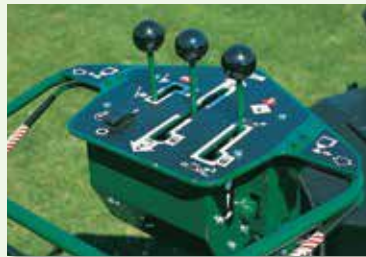
A new control panel for operator convenience features forward and reverse, brakes and fingertip throttle control.
