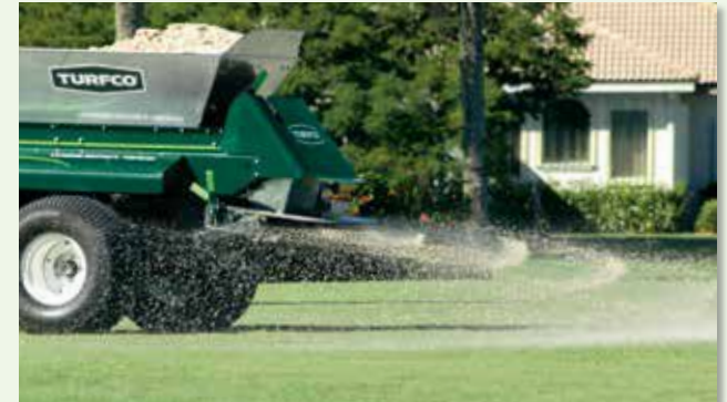
Adjustable spinner angled down for better turf penetration.
