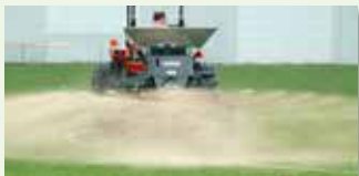
Adjustable spinner angles—up to 26° up or down.
