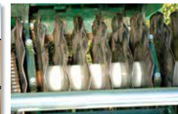
WaveBlade technology creates optimum clean slits, increasing seed-to-soil contact.
